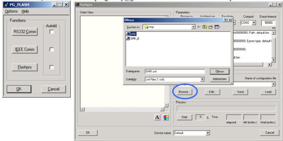
Open the configuration file dialog by pressing on the Browse button in the setup field. Select SMR, press the open button and confirm your selection with the Load button in the setup field. The Flashpro software updates all configuration settings according to your selection. You can select a different RS232 interface by choosing one of the COM-ports in the pulldown menu. Please do not change any other parameter. Then press Start to execute the update process:
