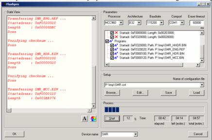
After the update process restart the SMR by switching the 'ON/OFF' button and click the Yes button to upload the reference oscillator value. Then start the internal calibration procedure described below.
