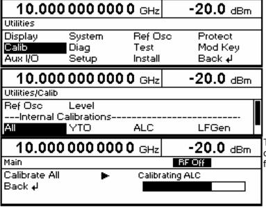
The SMR will start with the internal calibration procedure, which will take a few minutes.
